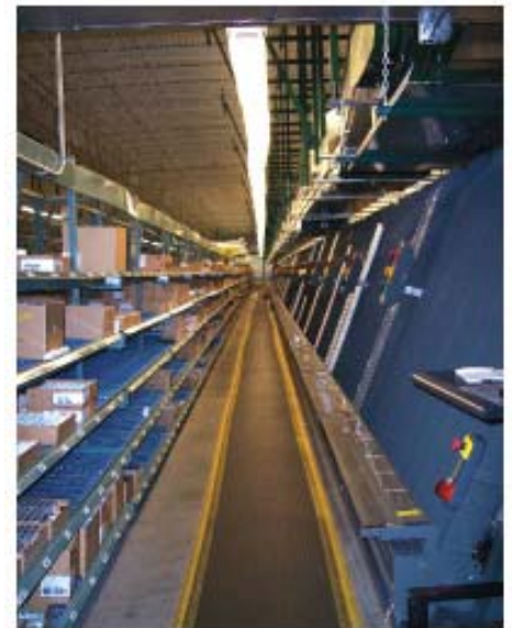
The A-frame dispenses 2,200 SKUs, mostly prescription and over-the-counter products.
