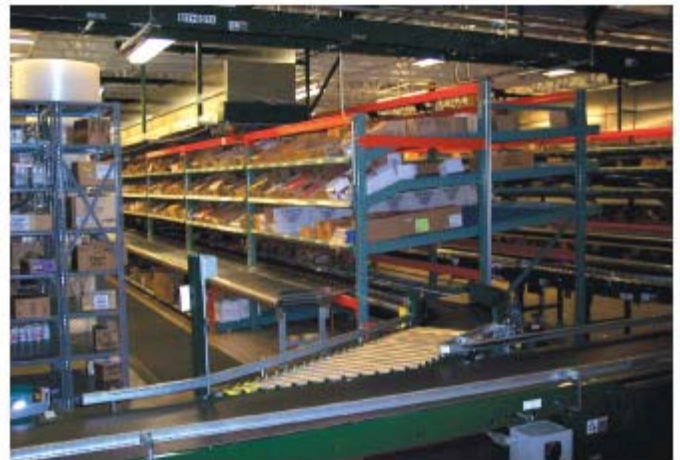
More than four miles of conveyor and sortation route product through the DC.
