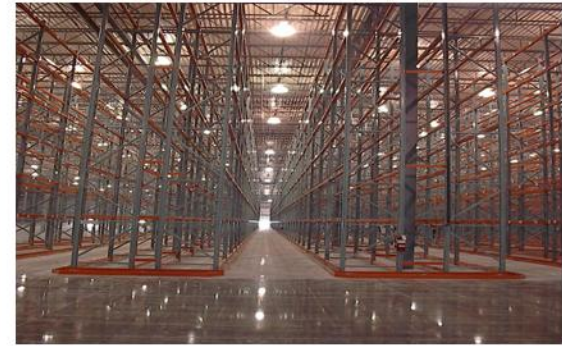
Hundreds of truck loads of selective racking were used in Harbor Freight DC's in South Carolina and California .
